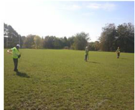
EM34 Single frequency Exploration depth up to 50m
