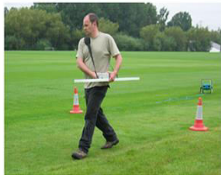
GEM-2 Multi-frequency Exploration depth up to 10m
