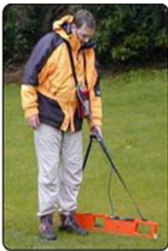
EM-38 Single frequency Exploration depth ~1.5m
